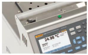
Fluid spills create mess and potential safety hazards. The 6109A and 7109A include an overflow tube that directs excess bath fluid into an optional overflow container. A drain tube makes it easy to remove bath fluid for replacement or transport.
